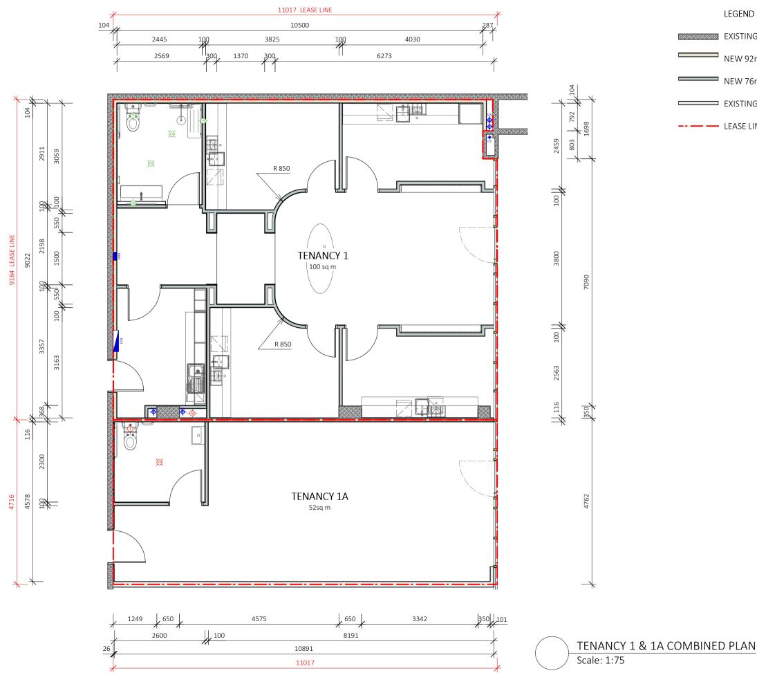
EXISTING TILT UP WALL NEW 92mm STUD WALL WITH 13mm PLASTERBOARD ■ NEW 76mm STUD WALL WITH 13mm PLASTERBOARD EXISTING IT STUD WALL WITH PLASTERBOARD - - LEASE LINE
